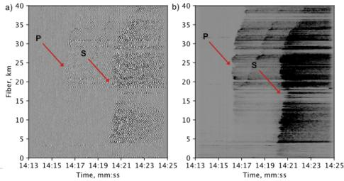
Figure 1 : Signals in time and distance from the beginning of the cable for the October 10, 2020 earthquakes. a) Represents the signals filtered between 5 and 30 Hz and b) their envelope.
